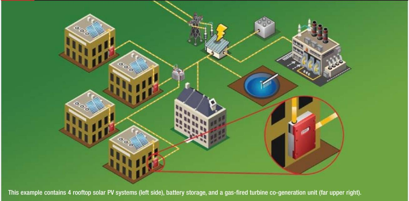
This example contains 4 rooftop solar PV systems (left side), battery storage, and a gas-fired turbine co-generation unit (far upper right).
