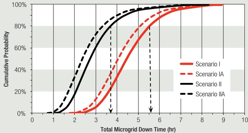
This analysis shows effect of summer storms on a microgrid located in Connecticut. The cumulative probability plots show the probability of downtime risk being less than or equal to a selected value (hours of downtime) on the horizontal axis. The Figure shows how an aggressive maintenance strategy (Scenario II, black curve) tends to reduce downtime risk as compared with a less aggressive strategy (Scenario I, red curve). The dotted-line curves show the effect of installing battery storage.
